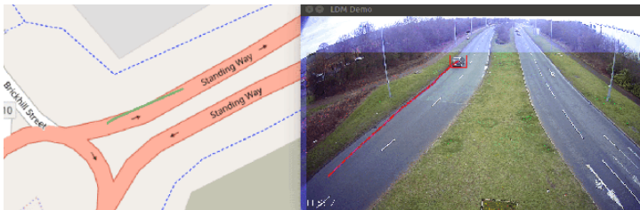
Vivacity Labs' sensors use computer vision and machine learning to process the activity on the roadway.
